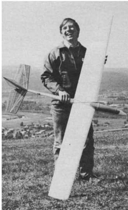
Dick Beltz and his two-meter Wizard, an original design that fought bigger ships tooth and nail. The 72-in. wing had 560 squares; 32 oz.
