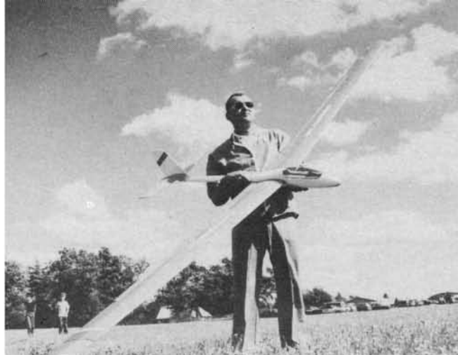
Bob Baugher and his Maestro, first-place winner on Saturday at Elmira. Sheeted wing with Grand Esprit airfoil. With a weight of 70 oz., the ship utilized elevator, rudder, spoiler, and flaperon controls.
